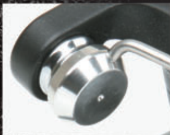
A single ball bearing is encapsulated within the line roller. This reduces slippage between the line and roller which, coupled with the slow oscillation, reduces line twist and wear on the monofilament.
